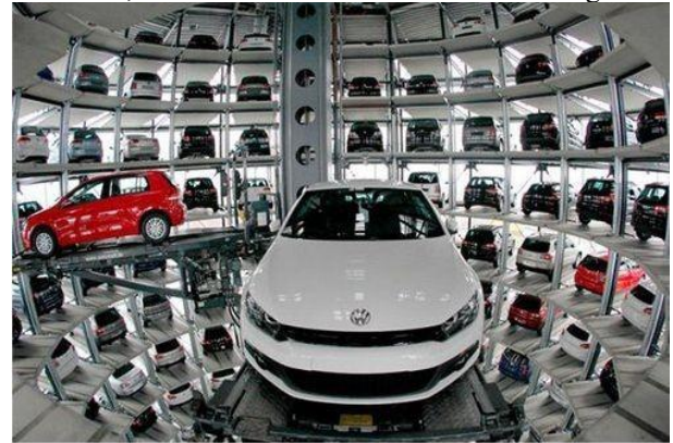
Fig.4 Mechanical parking lot
