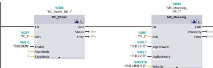
FIGURE 12 MOTOR 2 ENABLES FORWARD AND REVERSE ROTATION CONTROL
