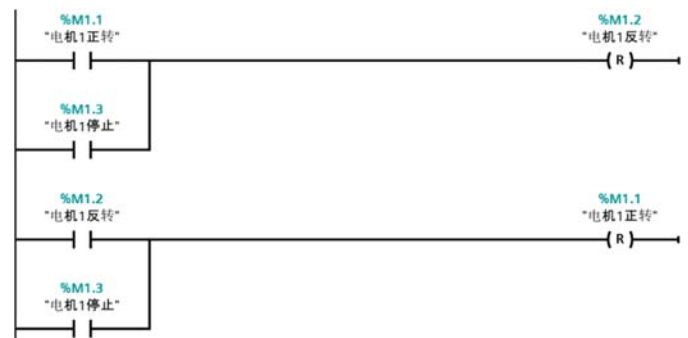
FIG.8. MOTOR 1 FORWARD AND REVERSE ROTATION AND STOP CONTROL
