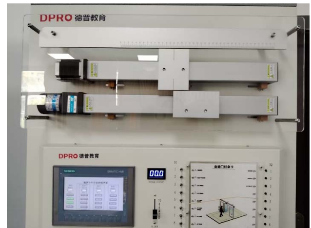
FIG.8 STEPPER MOTOR CONTROL TEST BENCH
